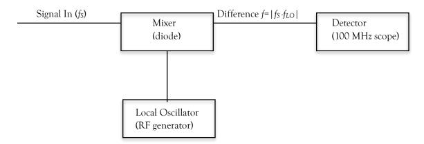
In order to look for such a signal it is convenient to supply an auxiliary "local oscillator" at a frequency very near the signal frequency and use a non-linear mixer to produce a intermediate signal at the difference frequency ( $|f_{LO}f_s|$ ). This lower "intermediate frequency" signal can be detected by a relatively slow device (in our case an ordinary oscilloscope).
