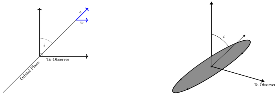
Figure 7: Side view (left) and three-dimensional visualization (right) of the relationship between orbital inclination and radial velocity. The circular orbit, shown in gray in the right image, is inclined by i degrees from the plane of the sky.
