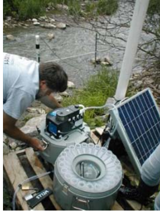
Fig. 2a. Servicing “R 2 D 2 ” the Teledyne ISCO automated water sampler located at the Rt 38A site. It collected 1-liter of water daily (4 am).
