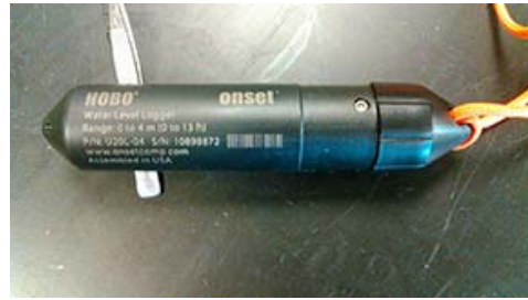
Fig. 2b. An ONSET HOBO U20L-004 data logger. Each pair of data loggers measured hourly water and air pressure to calculate hourly stream stage (height), and air and water temperatures.
