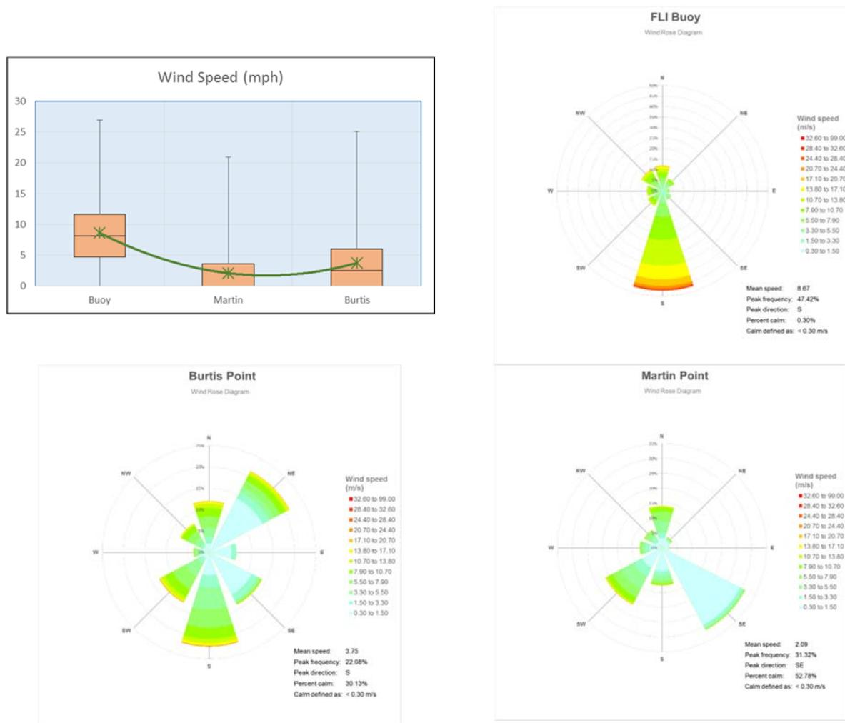
Fig. 25. Box and Whisker plots of wind speed (upper left) and wind roses from the FLI Buoy (upper right), Burtis Pt (lower left) and Martin Pt (lower right) over the deployment.
