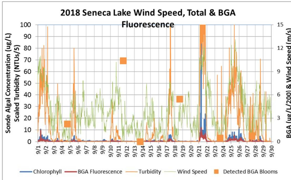
Fig. 19. Water turbidity, total and BGA fluorescence measured at a dock in Emerson Cove, Seneca Lake by an YSI EXO2 sonde. BGA concentrations at this site were from the Seneca HABs Surveillance team (with permission). Wind speed was measured by the Seneca Lake monitoring buoy, just offshore of this shoreline location.
