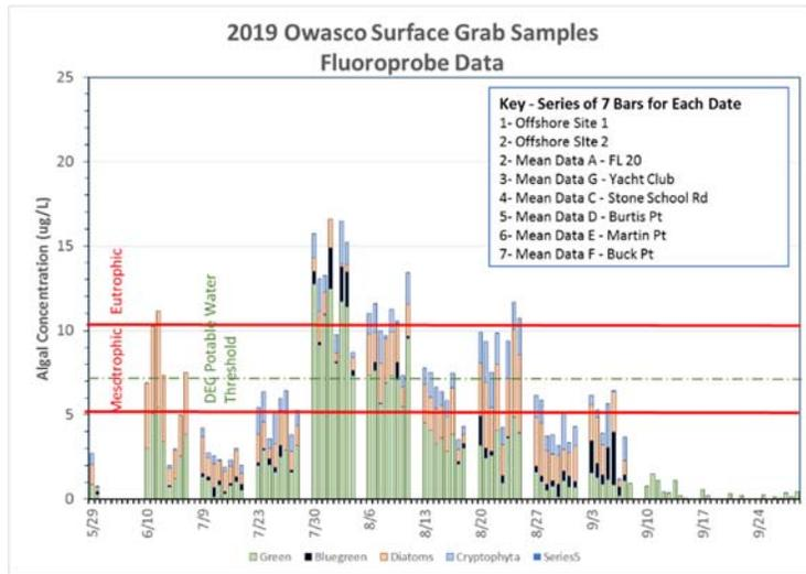
Fig. 8. bbe FluoroProbe grab sample data from each site (mean surface concentrations from Sites 1&2, and nearshore sites A, C-G) on each survey date. The dock surveys started on 6/10.
