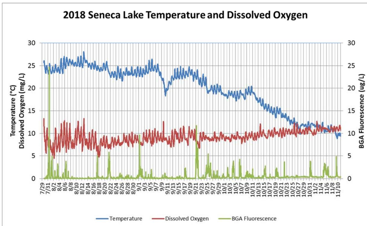
Fig. 22. Seasonal deployment of an YSI EXO2 Sonde in Seneca Lake that also revealed daily oscillations and co-variance of water temperature and dissolved oxygen concentrations.
