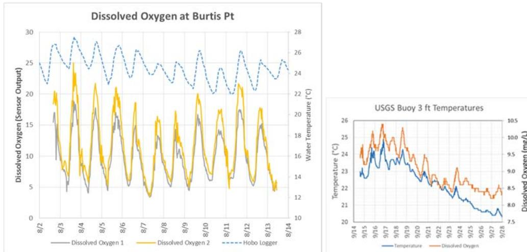
Fig. 21. Dockside FLI Sensor Node duplicate dissolved oxygen concentrations co-varied with the HOBO water temperature at Burtis Pt (left). The FLI Sensor Node dissolved oxygen output was not calibrated. Similar results were observed at Martin Pt. and at the USGS Buoy in September, 2018 (3-ft surface water sensor, right).
