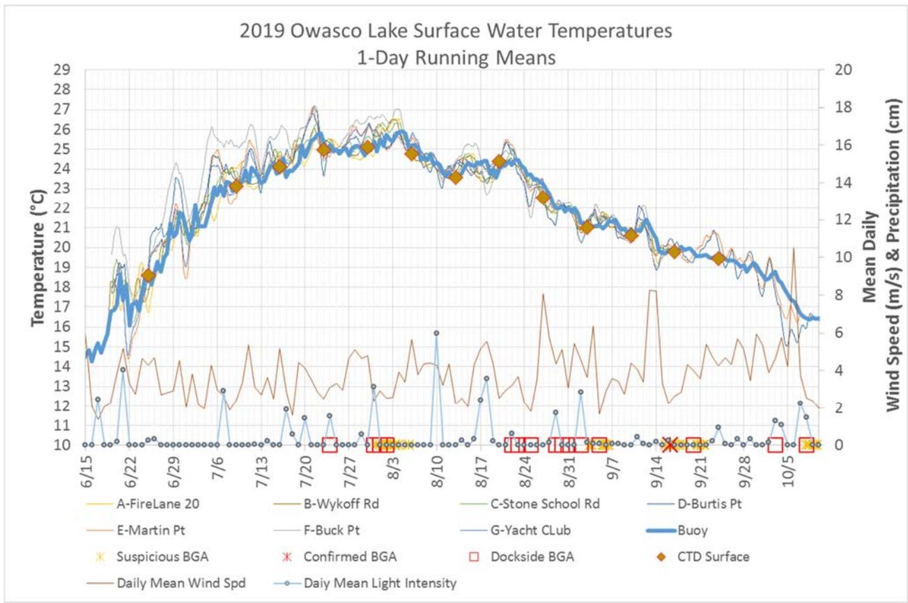
Fig. 18. Plot of nearshore and buoy 1m water temperatures, nearshore BGA suspicious, confirmed and dockside blooms, rainfall and mean daily wind speeds.
