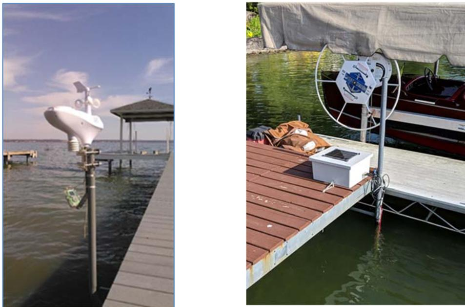
Fig. 4. A weather station (upper white instrument), automatic camera (green box) attached to a dock (left), and the FLI Sensor Node (grey box) with solar panel deployed in the field (right). The Node's sensors were tied to the dock leg.
