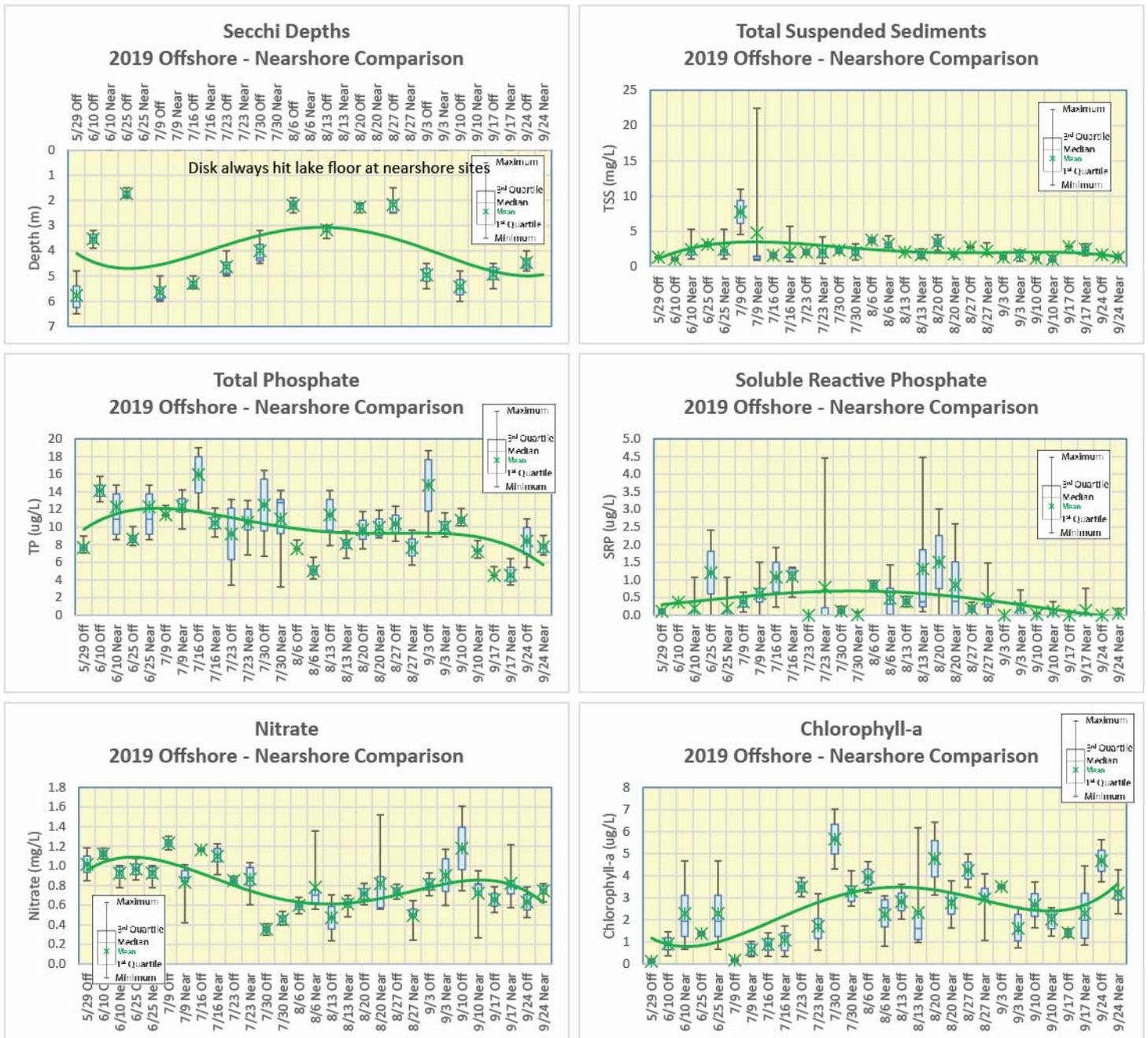
Fig. 9b. Nearshore to offshore site temporal comparison of the limnological data.
