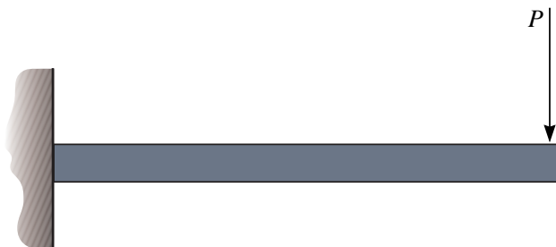
Figure 12 A cantilever held by a wall at one end and loaded at its free end.
