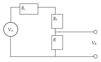
inductor just cancel. At that frequency the circuit reduces to a simple resistive voltage divider as shown in the diagram. (Here I have explicitly shown the output resistance of the signal generator,  $R_s$ ). With the scope you can measure the measure the voltage across  $R_h$  and R combined on one channel and across R alone on the other.
