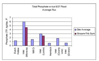
Fig. 22. Site averaged total phosphate flux.
