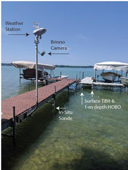
Fig. 3. Brinno camera, Weather station, and logger/sonde deployments at a dock (right). The *In-Situ sondes* and a temperature logger (*HOBOS*) were placed inside separate PVC pipes and strapped to a dock leg. The pipes protected the instrumentation from waves.
