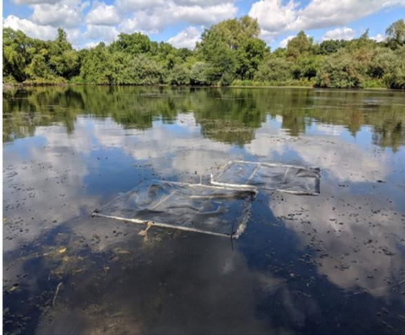
Fig. 4a. Mesocosm racks floating in a pond at Hanley Preserve (above right). Incubations were conducted in a small pond at the HWS Hanley Preserve to reduce the likelihood of losing or breaking a rack due to waves and winds in Owasco Lake. Temperature and solar radiation measurements were made at the site every five minutes during the five-day incubation.
