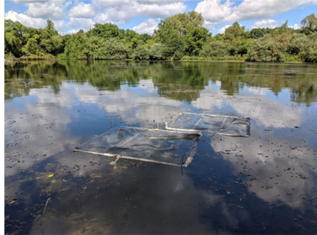
Fig. 4. Mesocosm racks floating in a pond at Hanley Preserve. Incubations were conducted in a small pond at the HWS Hanley Preserve to reduce the likelihood of losing or breaking a rack due to waves and winds in Owasco Lake. Temperature and solar radiation measurements were made at the site every five minutes during the five-day incubation.
