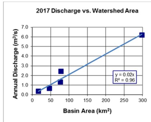
Fig. 18. Discharge vs. Basin Size.
