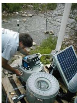
Fig. 4a. Servicing “R<sub>2</sub>D<sub>2</sub>” the Teledyne ISCO automated water sampler located at the Rt 38A site. It collected 1-liter of water daily (4 am) and was serviced every one to two weeks.
