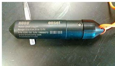
Fig. 4b. An ONSET HOBO U20L-04 data logger. Each pair of data loggers measured hourly water and air pressure to calculate hourly stream stage (height), and air and water temperatures.
