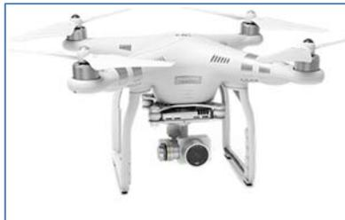
Fig. 3. The drone used in this study, a Phantom 3 Advanced by DJI.
