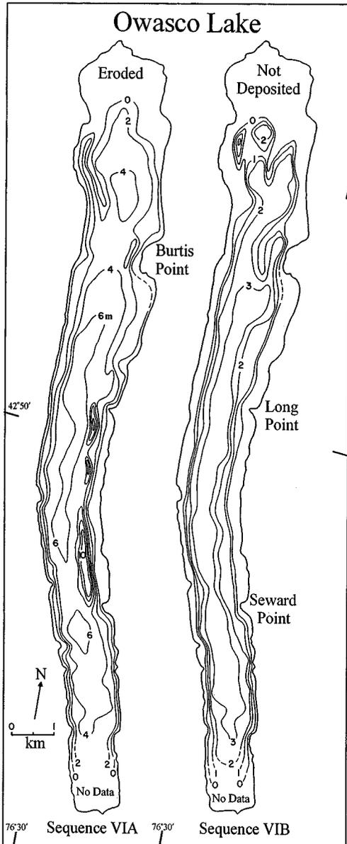
FIG. 4. Isopach maps of seismic sequences VIA (left) and VIB (right) in Owasco Lake.
