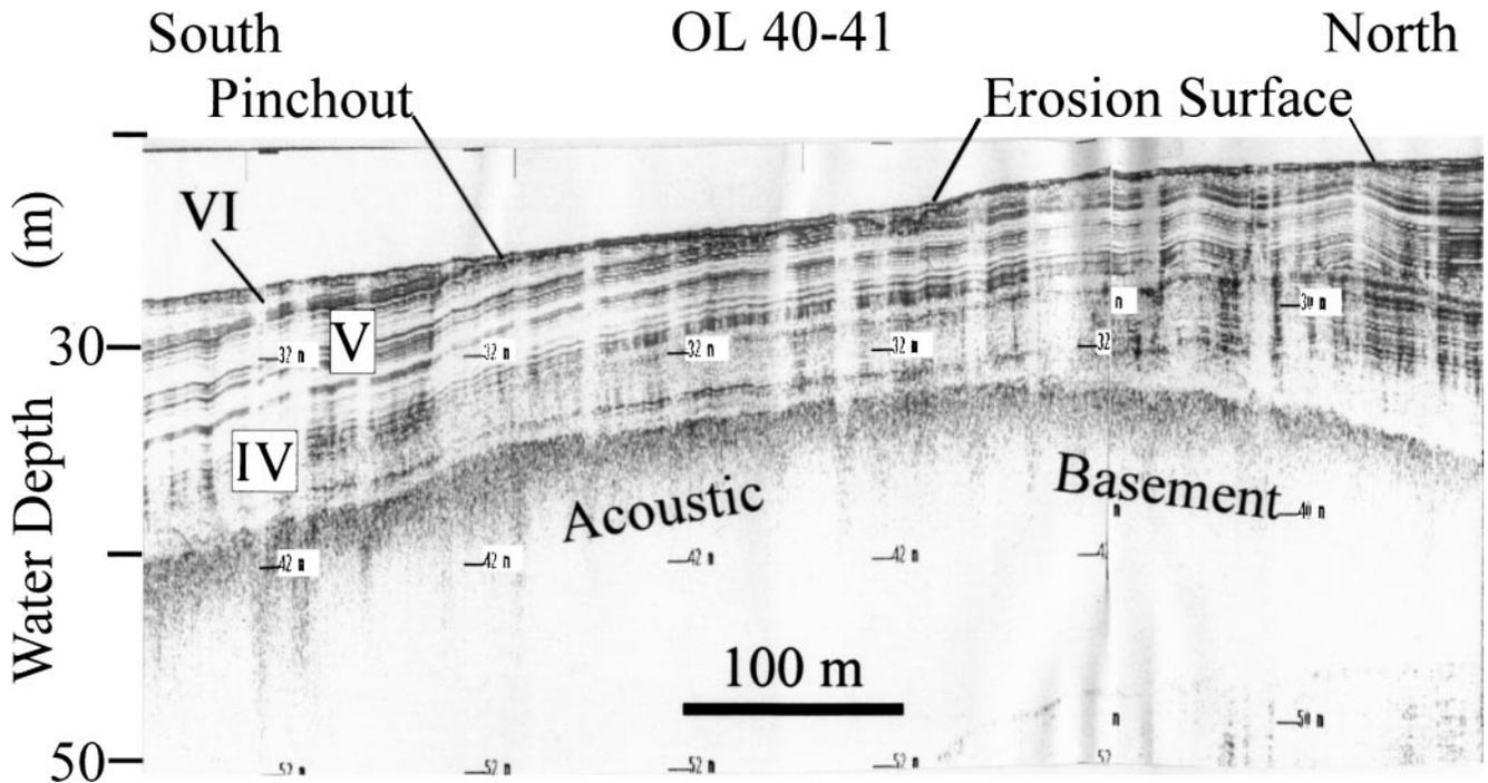
FIG. 7. North part of axial seismic reflection profile 40–41 (Fig. 2) illustrating pinchout (onlap) of sequence VI against erosion surface that truncates reflectors in sequence V.
