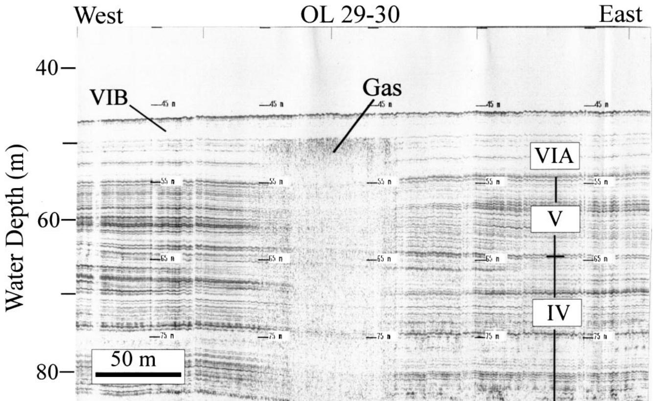
FIG. 9. Central part of seismic reflection profile 29-30 (Fig. 2) illustrating a "seismic smear" interpreted as biogenic gas concentrated along the sequence VIA/VIB boundary.
