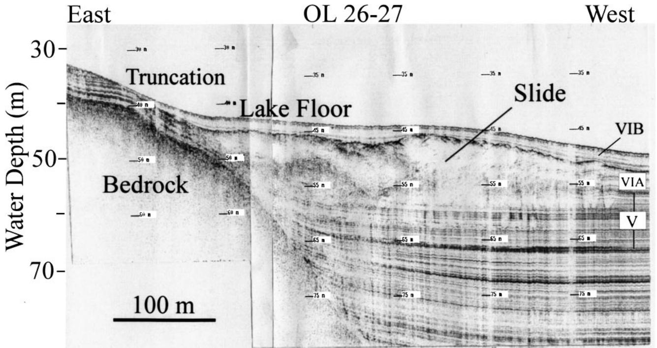
FIG. 6. Part of seismic reflection profile 26–27 (Fig. 2) illustrating subaqueous slide deposit at or near the sequence VIA/VIB boundary.
