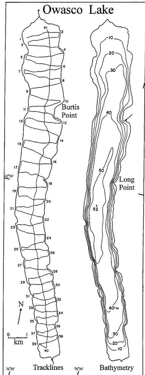
FIG. 2. Seismic reflection tracklines (left) and bathymetry (right) of Owasco Lake.
