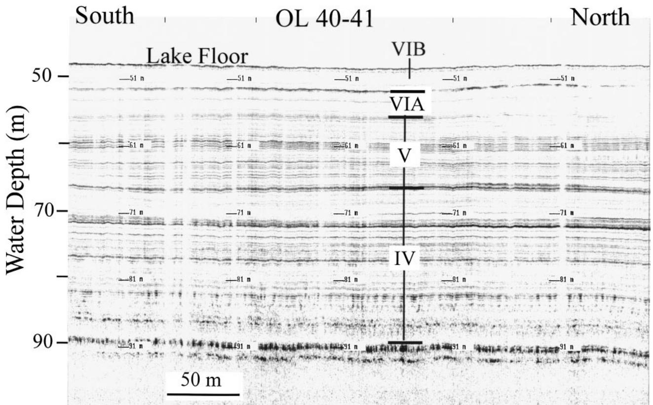
FIG. 3. Part of seismic reflection profile 40–41 (Fig. 2) illustrating depositional sequences VIA and VIB.
