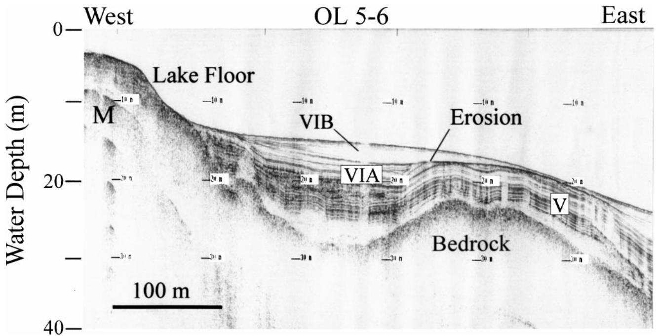
FIG. 8. Western part of seismic reflection profile 5-6 (Fig. 2) illustrating erosion surface along the sequence VIA/VIB boundary. This position implies a middle-Holocene age for the start of erosion. M indicates multiple reflection.
